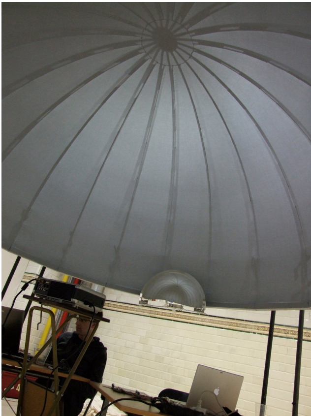
Figure 3: First Méta-crâne hardware prototype, designed and realized by Thomas Israel and Thierry Sablon, featuring a video projector and a spherical mirror
